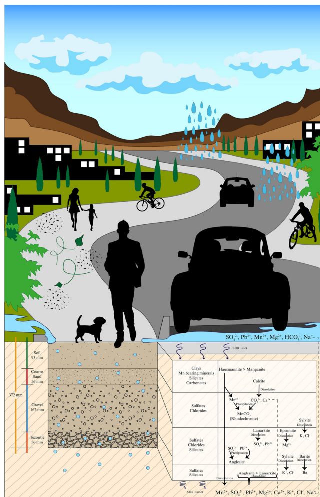
Fig. 5. Geochemical modeled interactions between urban runoff pollutants and the filter materials.
