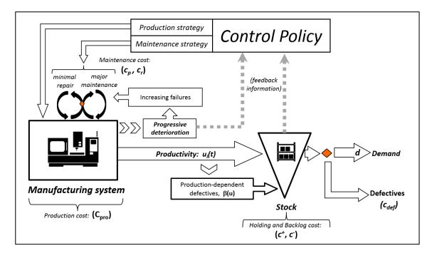
Figure 1. Manufacturing system under study.
