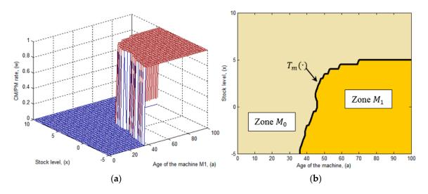
**Figure 6.** Repair/major maintenance switching policy. (**a**) Repair/major maintenance rate; (**b**) Trace of the repair/major maintenance policy.
