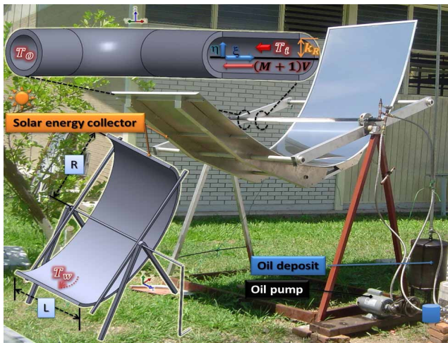
Figure 4. Solar concentrations for hot oil of the interchange.
