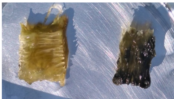
Fig. 3. Immobilized mycelium of Cladosporium cladosporioides in Luffa cylindrica , before and after the secretion of a pigment.
