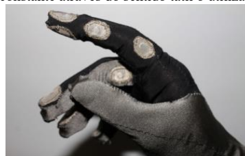
Figura 2 Luva Argot (A Wearable One-Handed Keyboard Glove)
