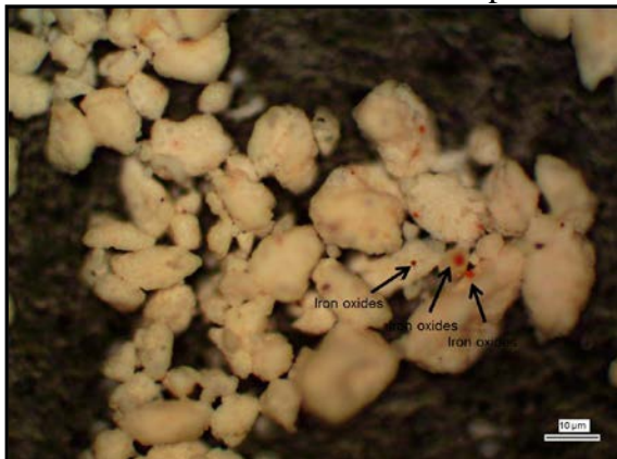
Figure 1 General image of sample of kaolin mineral (100x, Optical Microscopy)
