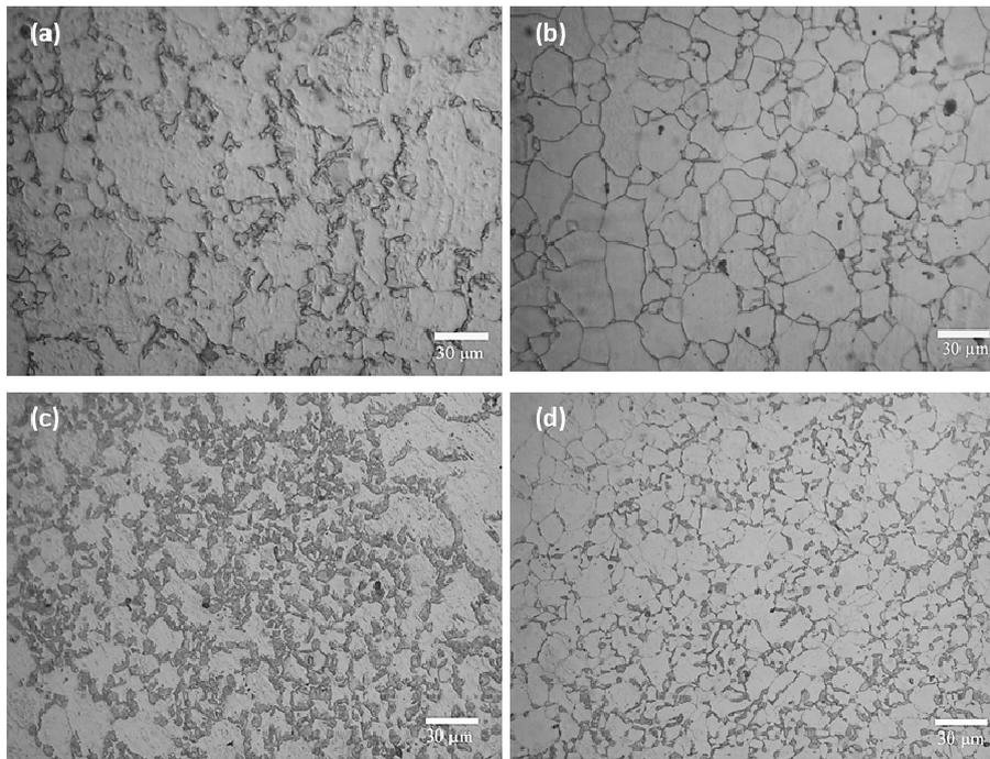
**Fig. 3** Micrographs of the DP steels intercritically treated at: **710°C** - a) DP1(0.00%Ti), b) DP3 (0.05% Ti) - and at **720°C** - c) DP1 (0.00% Ti), and d) DP3 (0.05% Ti).
