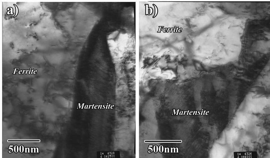
Fig. 4 TEM micrographs of the 720°C treated steel containing 0.06%Ti
