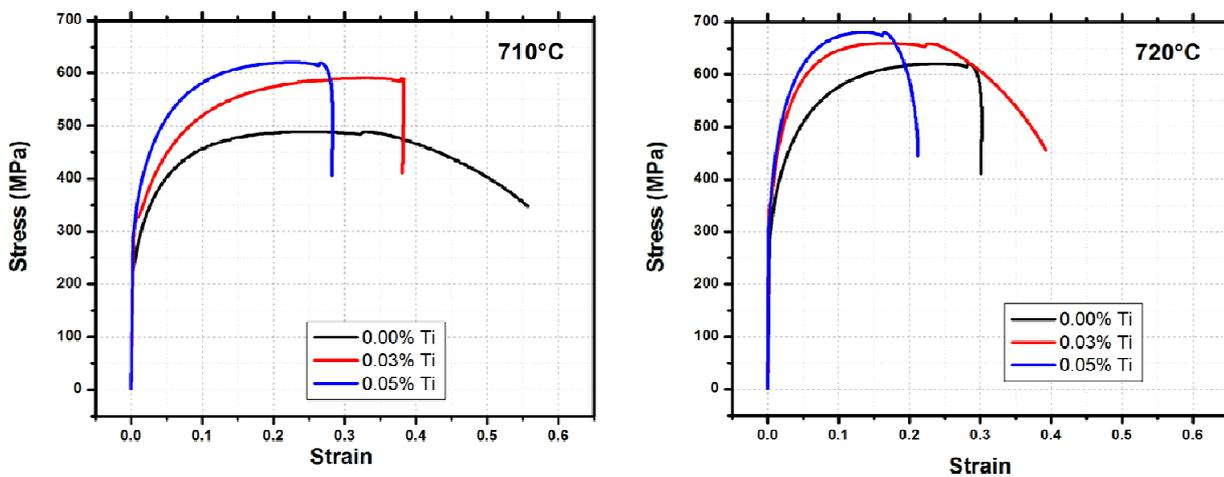
Fig. 6 Stress - strain curves for the DP steels
