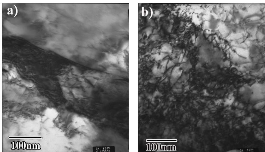
Fig.7 TEM micrographs showing the difference in dislocation density for the DP1 steel (a) and for the DP3 steel (b).
