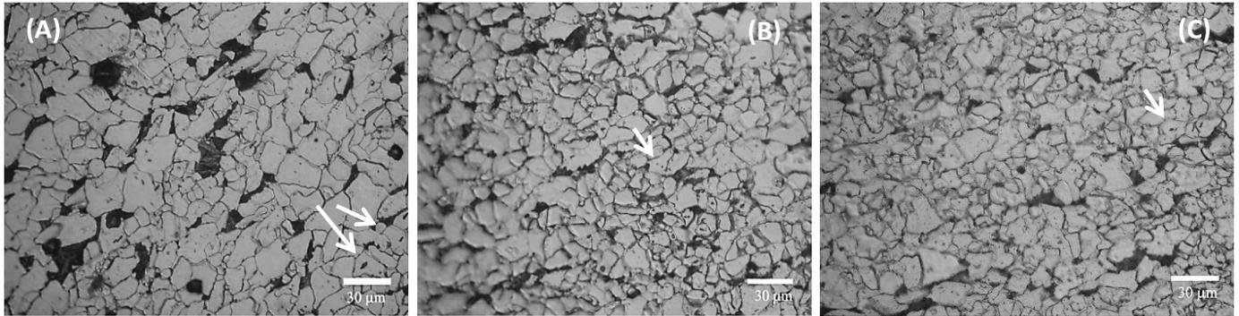
**Fig. 1** Optical microscopy of the DP steels after the thermomechanical treatment: (a) base DP1 steel, (b) 0.03%Ti DP2 steel, and (c) 0.05% Ti DP3 steel.
