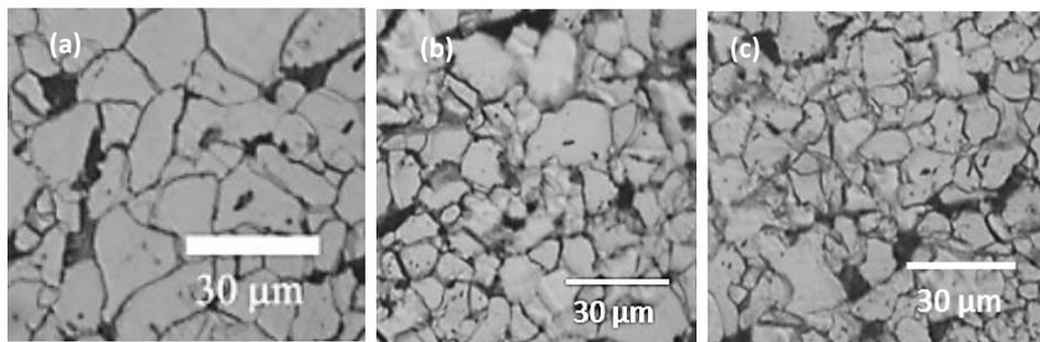
**Fig. 2** Pearlite islands formed in the center of the ferrite grains, a) base DP1 steel, b) 0.03%Ti DP2 steel, and c) 0.05%Ti DP3 steel.
