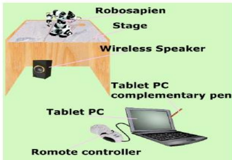
Figure 3. Components of at-site controlled robot (Zhen-Jia et al, 2006)
