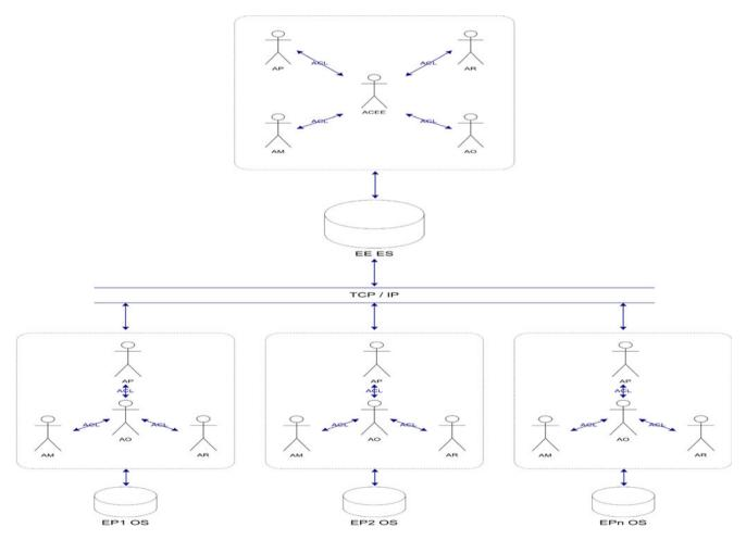
Fig. 5 Structure of the MAS for the extended enterprise
