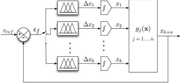
Fig. 1. Fuzzy control for optimizing the circuit design.
