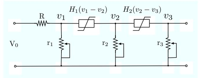
Fig. 6. Non-linear passive circuit.
