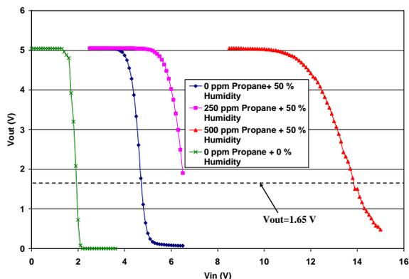
Figure 5. Experimental transfer functions, as a result of chemical reaction of the sensing layer with propane, in the presence of 50 % of humidity inside the test chamber.
