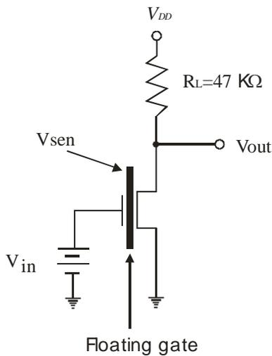
Figure 2. Amplifier used to model gas sensing with an FGMOSFET.
