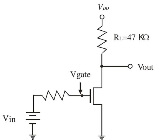
Figure 4. Experimental amplifier configuration, using a conventional MOSFET.
