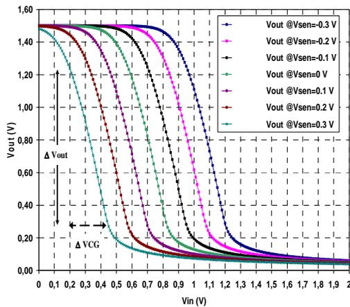
Figure 3. Transfer function of the amplifier used for the theoretical analysis of gas interaction of a sensing layer in contact with the floating gate of an FGMOSFET.  $W_n/L_n=12\mu\text{m}/1.6\mu\text{m}$ .
