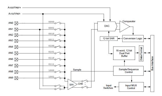
Figure 1. 12-Bit ADC Functional Block Diagram.
