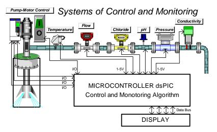
Figure 3. Systems of Control y Monitoring by Corrosion.
